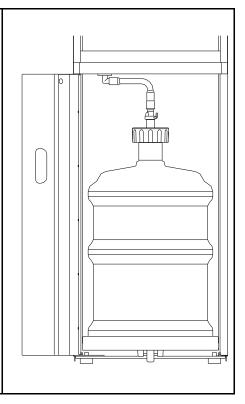
NOTE: If there is not a secure connection between the hose cap and the connector on the water cooler, the water pump will operate but the water cooler will not dispense water. Make sure the hose is connected to the water cooler correctly.
